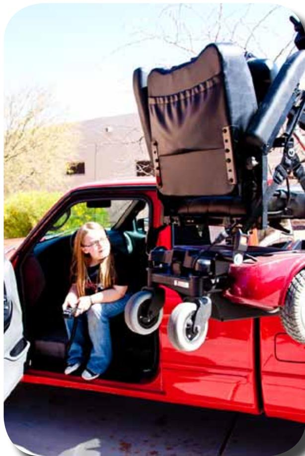
And of course Carol picked out a red one! The fully powered Bruno Outrider lift is operated by a remote control which Carol will use from the drivers' side. A seat cushion and petal extensions are custom made to fit Carol's height and leg length. A small box is made for her feet to rest on so that her legs aren't dangling. Two hand rails are installed to help her navigate into the driver's seat.
